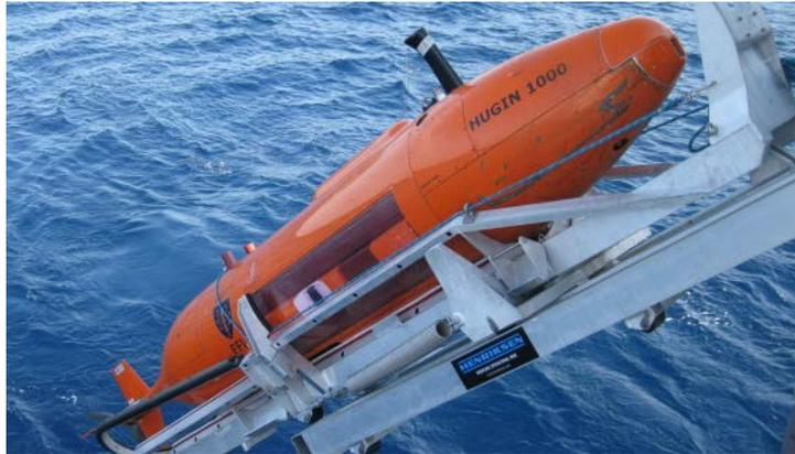
*Fig. 1: Norwegian Defence Research Establishment's HUGIN AUV equipped with a HISAS 1030 SAS system (60-115 kHz) and an added prototype low frequency transmitter (12-38 kHz)*
